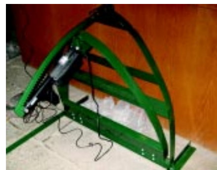
Clerestory windows — trial mechanism
